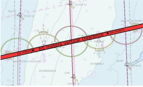
Note that only some of the bridge span in the TSS have 65 meters of vertical clearance. Ships with air draught more than 64 meters are to pass the TSS near the centreline. More information can be obtained at the Great Belt VTS
